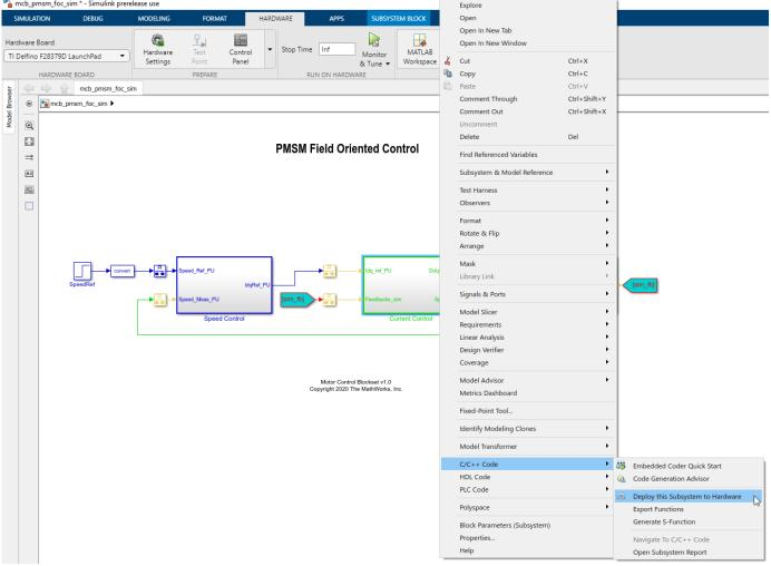
The system displays the  ${\bf Build\ code\ for\ Subsystem\ }$  dialog box. Set the Storage Class to Inlined for all parameters.
