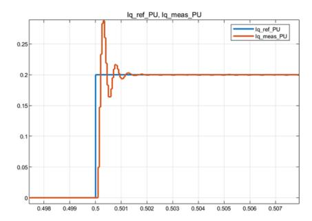
Follow the same procedure for the Id\_ref current to tune the *d*-axis current controller. After tuning both current controllers, set the **Mechanical input configuration** parameter, in the Surface Mount PMSM block parameters dialog box, back to Torque.
