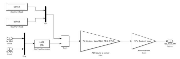
This subsystem reads the current in ADC counts and converts it to per-unit (PU) values.
