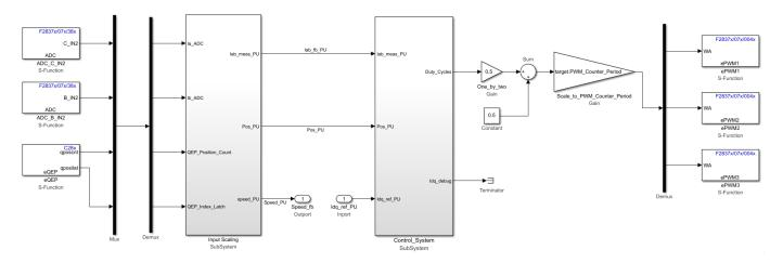
For simulation, add a variant source/sink to the hardware driver block for simulation and code generation.
