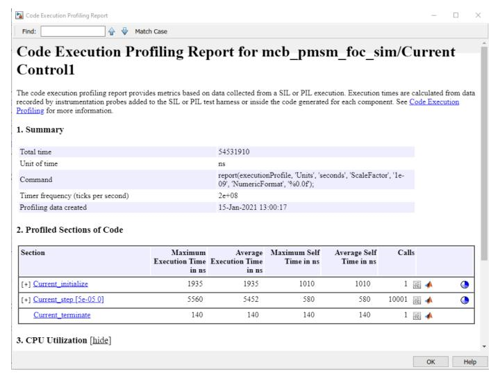
This profiling report, which is for the fixed-point datatype, shows the maximum and average execution times of the Current Control (PIL) subsystem running on the target hardware.
