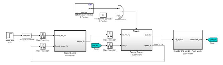
Simulate the model with the updated driver blocks and check the simulation results in the Simulation Data Inspector. Variants ensure that ADC, PWM drivers, and interrupts are not active during simulation.
