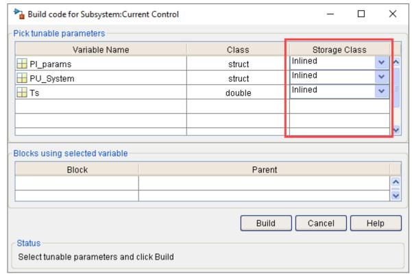
6 Click **Build** to create a model named untitiled that includes a PIL subsystem called Current Control.
