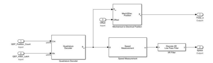
This subsystem reads the rotor position from the QEP pulse count.
