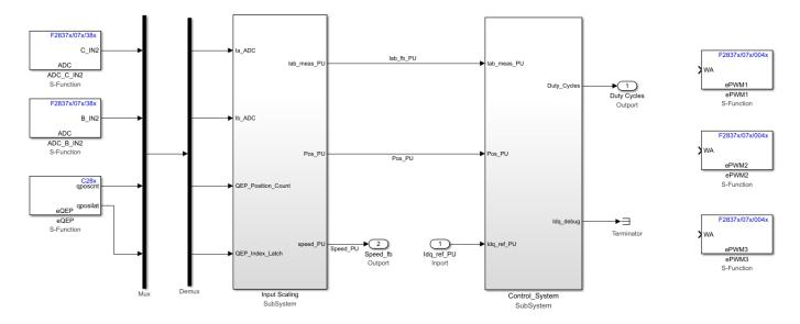
The ePWM blocks expect the duty cycle value to range from 0 to the PWM counter period value (5000). The Control\_System subsystem outputs the PWM in the range -1 to 1. The model needs to scale the output to 0 to 5000 (PWM counter period value).
