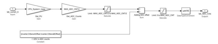
The maximum measurable peak current is considered as the base current. The ADC counts can be calculated from the base current and full-scale ADC values, along with the ADC offset, by using this equation:
