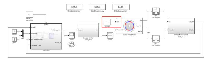
Simulate the model and plot the  $Iq\_ref\_PU$  and  $Iq\_meas\_PU$  current signals and analyze the step response. This helps you to tune the control parameters for the q-axis current controller to meet the control objectives.
