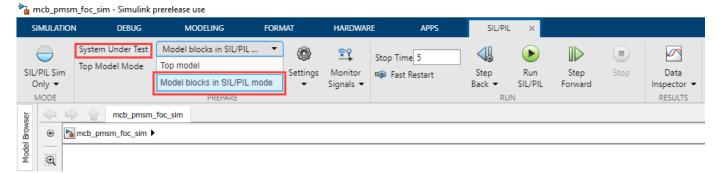
Click **Run SIL/PIL** on the **SIL/PIL** toolstrip to build the Current Control (PIL) subsystem and deploy it to the target.
